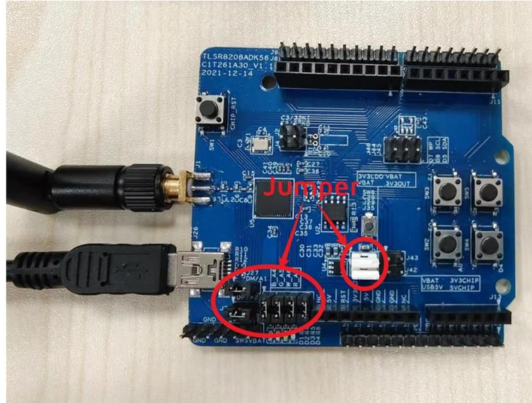
**Figure 2-2 USB to LDO 3.3V power supply**
